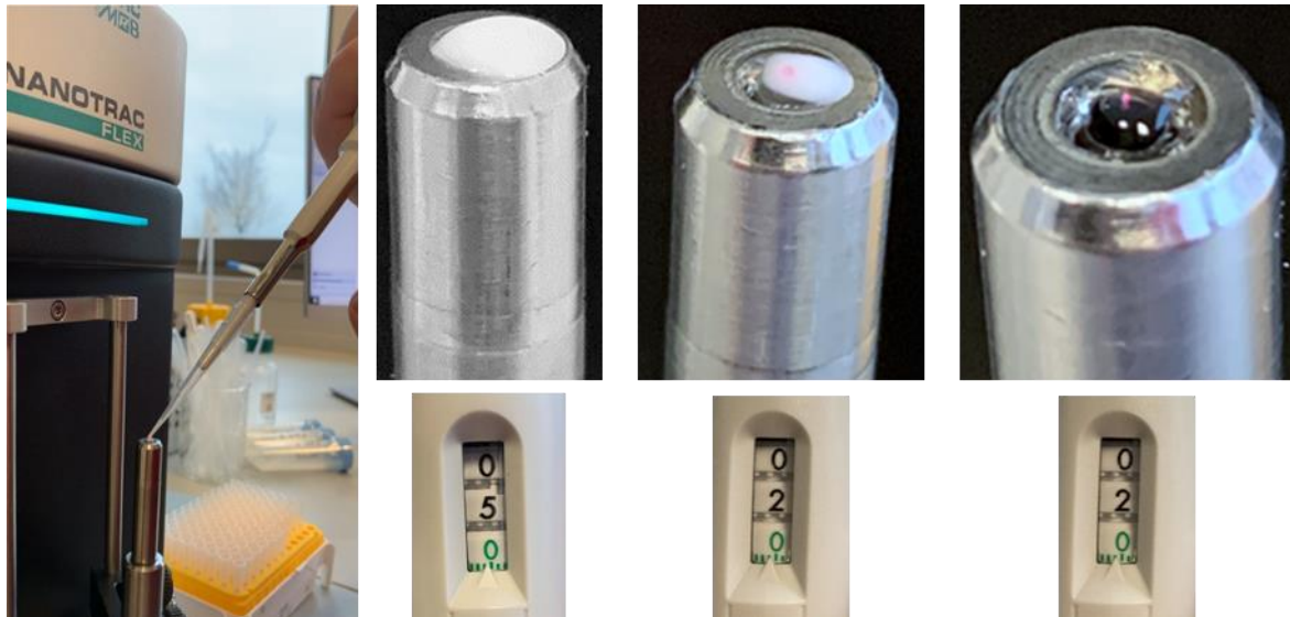
Figure 6: The sample is directly applied to the tip of the upside-down probe. From left to right: 5 \mu\text{L} undiluted sample, 2 \mu\text{L} undiluted sample, 2 \mu\text{m} highly diluted sample.
